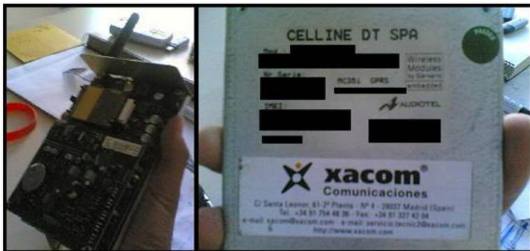
Its a GSM base station based on MC35i Siemens's module.
